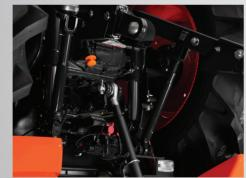
easier and increase lift capacity up to 4,378 pounds. Two external hydraulic lift cylinders make maintenance External Hydraulic Lift Cylinder
